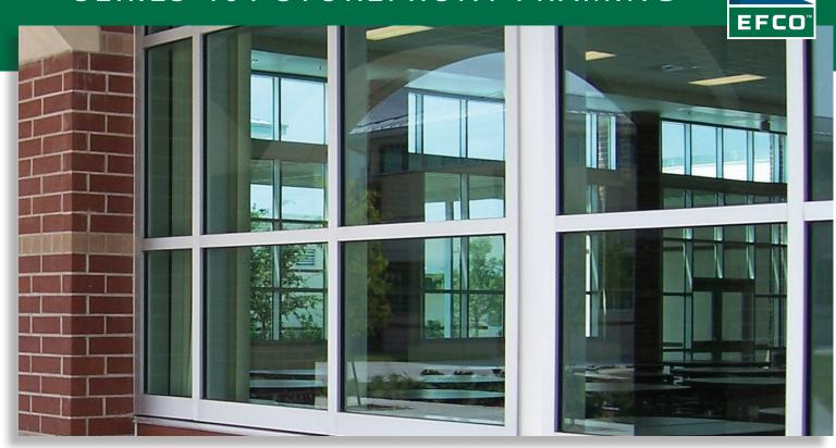
Shear Block • Screw Spline • Can Receptor Series 401 is an economical 1-3/4" X 4-1/2" flush glaze system available in both shear block and screw spline fabrication methods. Series 401 Storefront can accommodate all standard 1 3/4" and 2" entrances as well as WV410 vents. Vertical mullions will accept steel reinforcement to enhance structural performance.
